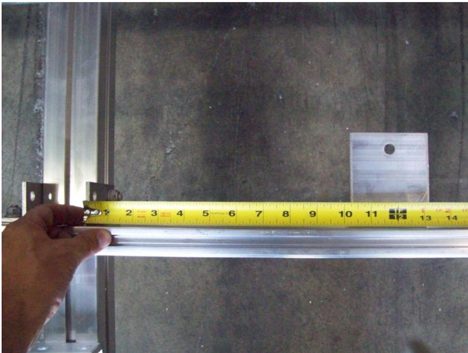
**Measure out 10 ¼" from the tongue to the edge of each mounting bracket. Position brackets then tighten nuts. Brackets can also be mounted on the rear crossbar and adjusted to accommodate different boxes.**
