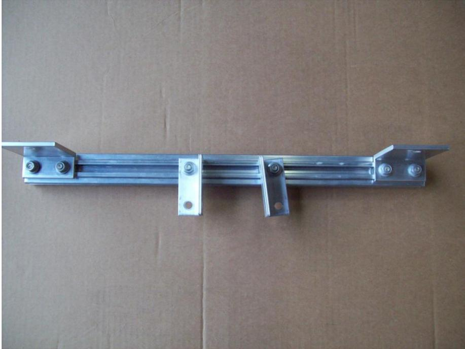
**Install the inner edge of the angle bracket on the 10 ¼” reference mark and tighten in place. Leave the other side loose for now**
