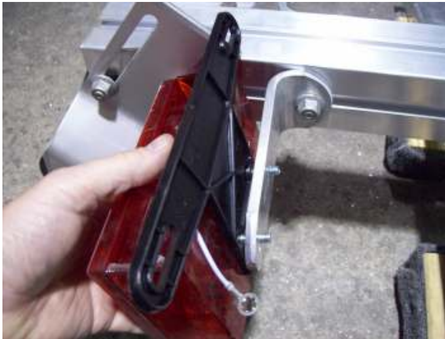
Trailer shown upside down Install the license plate bracket and left tail light onto the tail light bracket.
