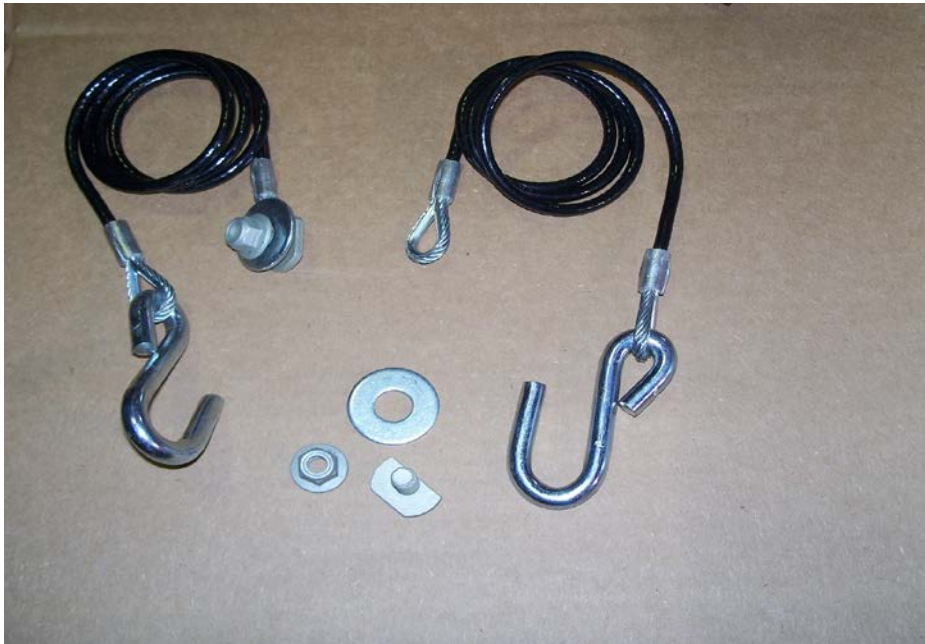
Safety hitch cables and hardware
