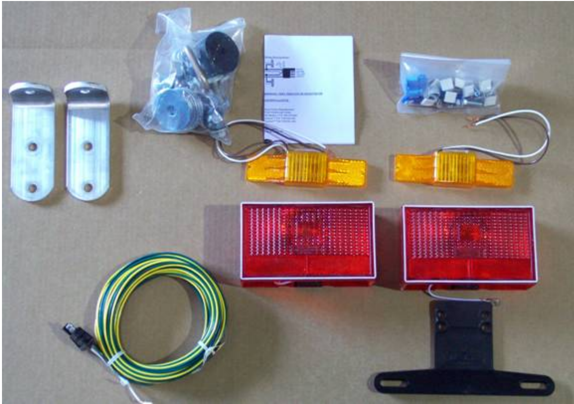
Lights, brackets, harness, and hardware
