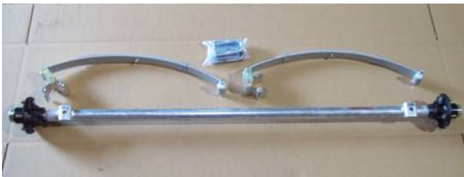
Axle assembly, springs and U bolt hardware.
